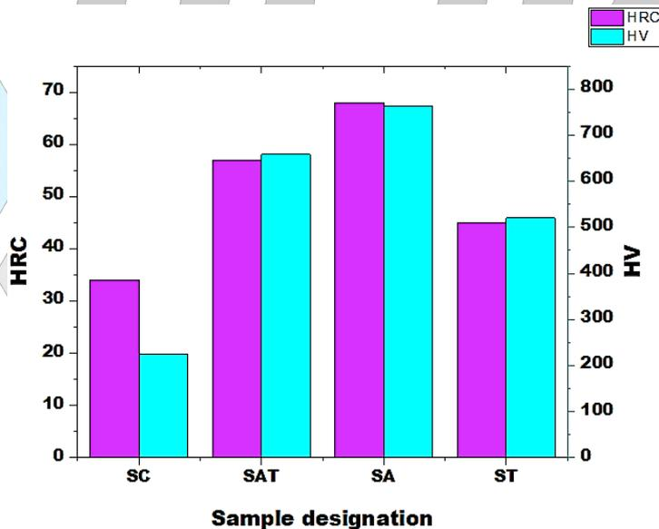
**Figure 3:** Effect of different tempering conditions on the Hardness of S7 Tool Steel
