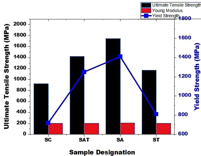
**Figure 2:** Effect of different tempering conditions on the Ultimate Tensile Strength, Yield Strength and Young Modulus of S7 Tool Steel
