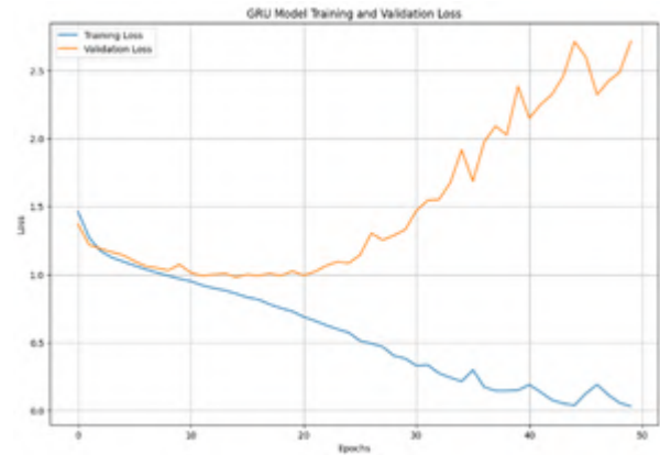
Figure 2. shows the Training and Validation Loss of the base model trained with an epoch of 50, Batch Size of 64, and 20% of Validation data.
