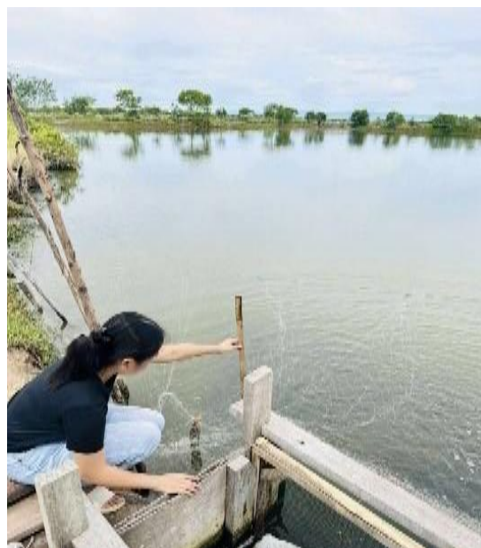
Figure 8: The bamboo pole is placed into the pond to measure the water's depth.
