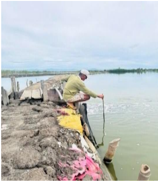
Figure 9: Marked bamboo sticks are inserted vertically into the pond to visualize water levels.
