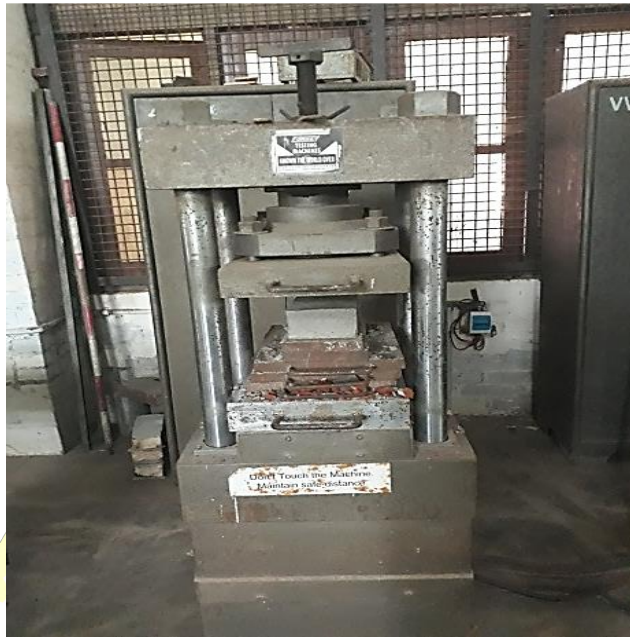
Figure 4. Compressive strength test of blocks
