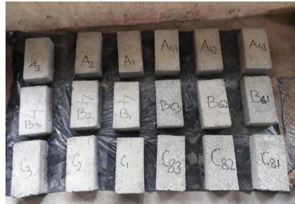
Figure 1. Freshly made cement-sand-gravel blocks.
