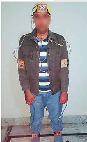
Figure 5: Ultrasonic sensors placed on various parts of the body for object detection [9].
