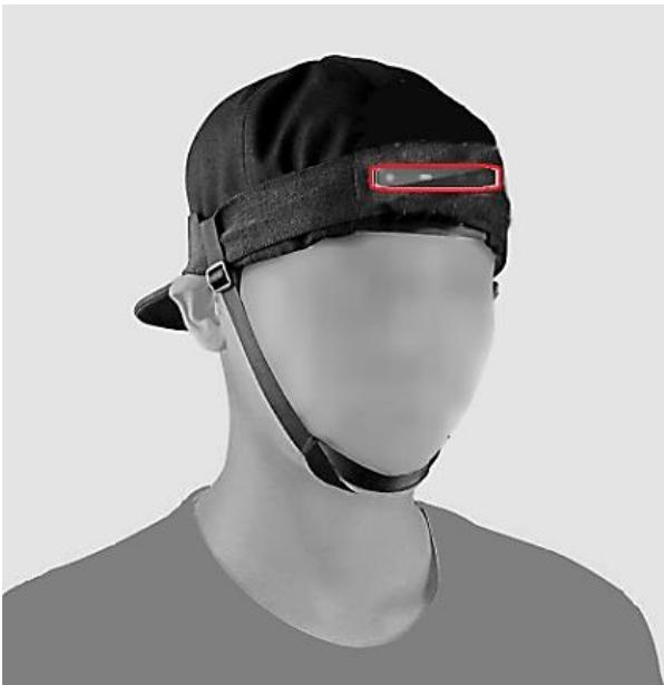
Figure 9: The depth camera implanted in a cap and placed on the head.
