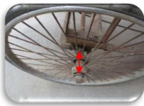
Photo 6: Small width of spoke span
