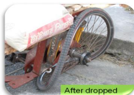
Photo 16. Drop test of the developed rickshaw van
