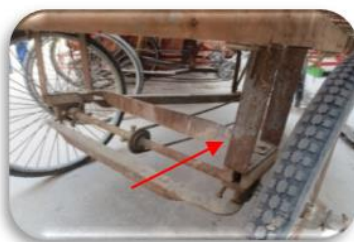
Photo 5: Platform support without suspension
