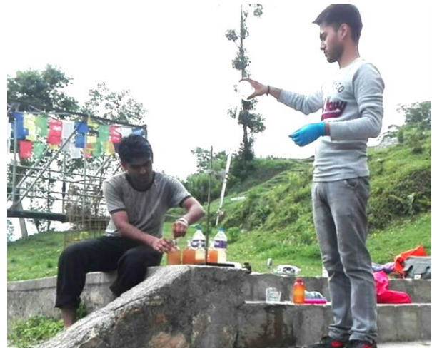
Figure 1: On-site analysis of Chloride and Dissolved Oxygen
