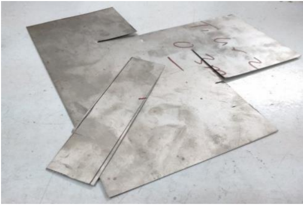
Figure 3.2 Ti of 0.3 mm thick sheet
