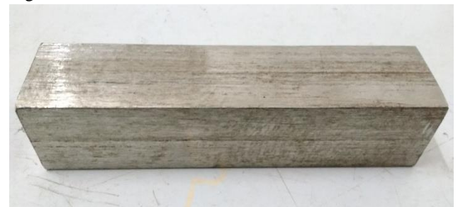
Figure 3.1 Machined specimen of AISI304 Stainless steel specimen
