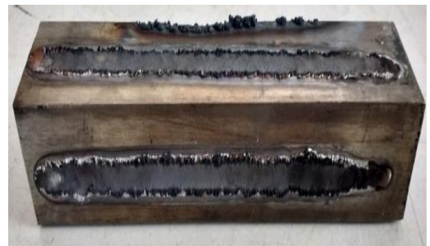
Figure 4.1 Ti surface alloyed AISI304 Stainless steel specimen
