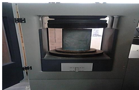
Figure 2: Specimen in Compressive Testing Machine
