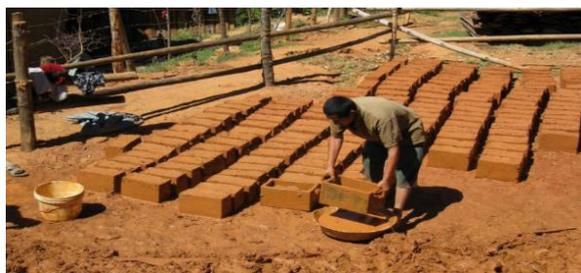
Figure 13: Bhutanese mud bricks (Bhutan Green Building Design Guidelines)
