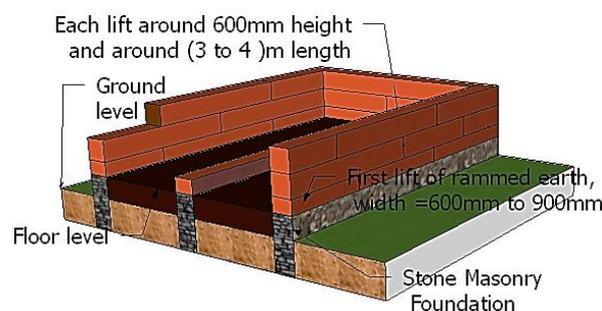
Figure 4: Construction configuration of rammed earth Walls and Foundation.
