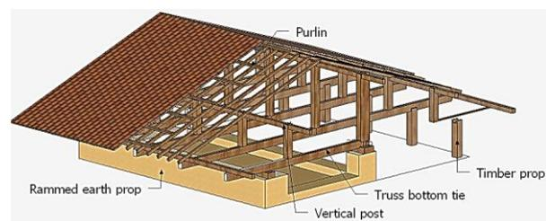
Figure 7: Layout of Traditional Roof truss and its elements
