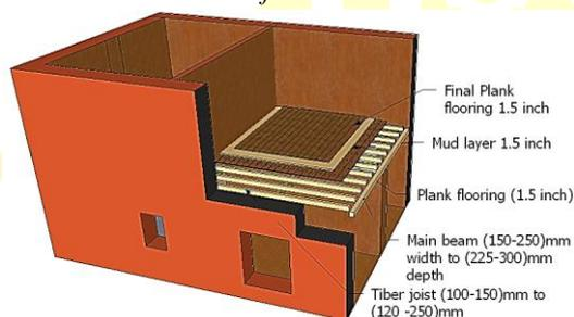
Figure 6: Floor joist and flooring configuration
